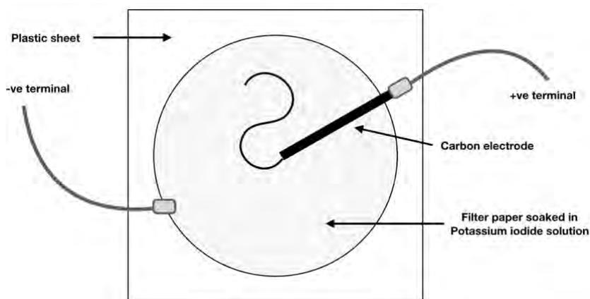
electrode of an electric circuit (attached to negative terminal of power source). For the other electrode, a carbon rod (carbon is electrically conductive) is used as a 'pen nib' to 'write' on the filter paper. When this electrode is made positive, the writing (brown iodine) is visible. If you reverse the polarity, the writing disappears.
